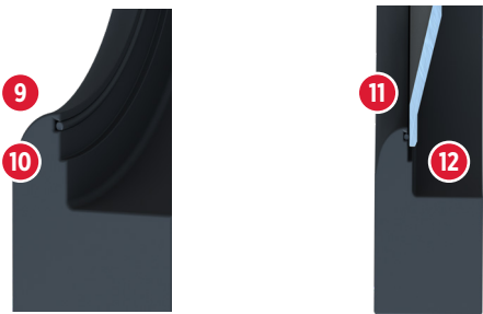
Figure 05: Integral Soft Seat Close-Up Cutaway Views.
