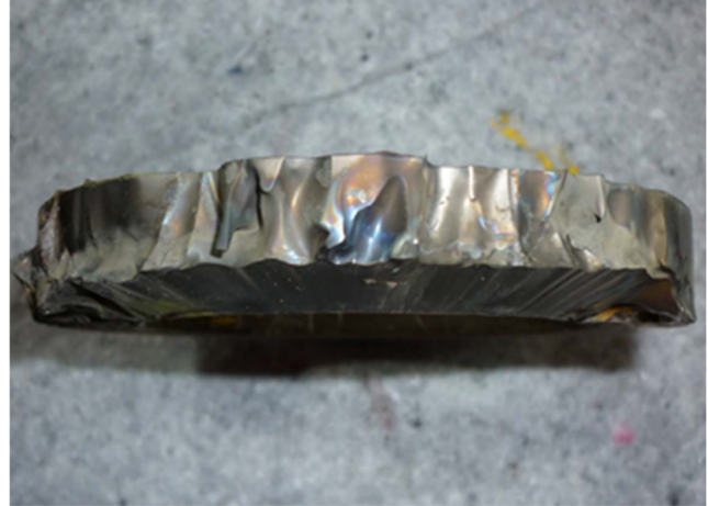
Erosion due to high velocity flow
