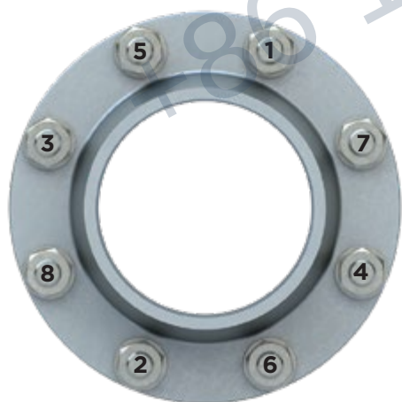
Figure 2 – Flange Bolt Tightening Pattern
