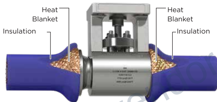
Figure 7: Insulation During PWHT Process
