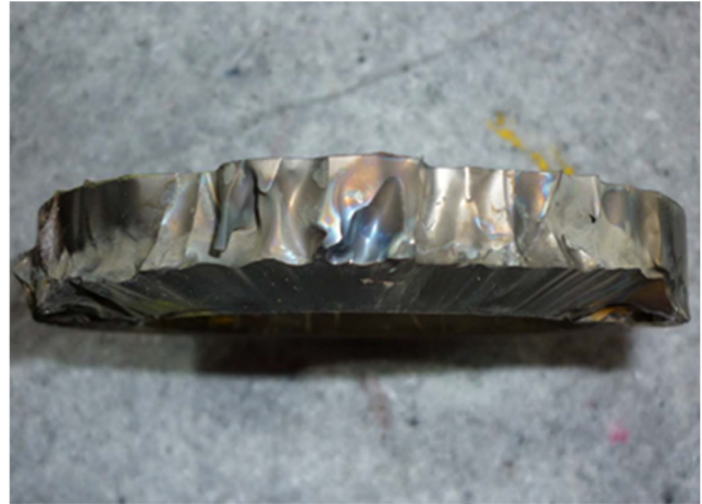
Erosion due to high velocity flow
